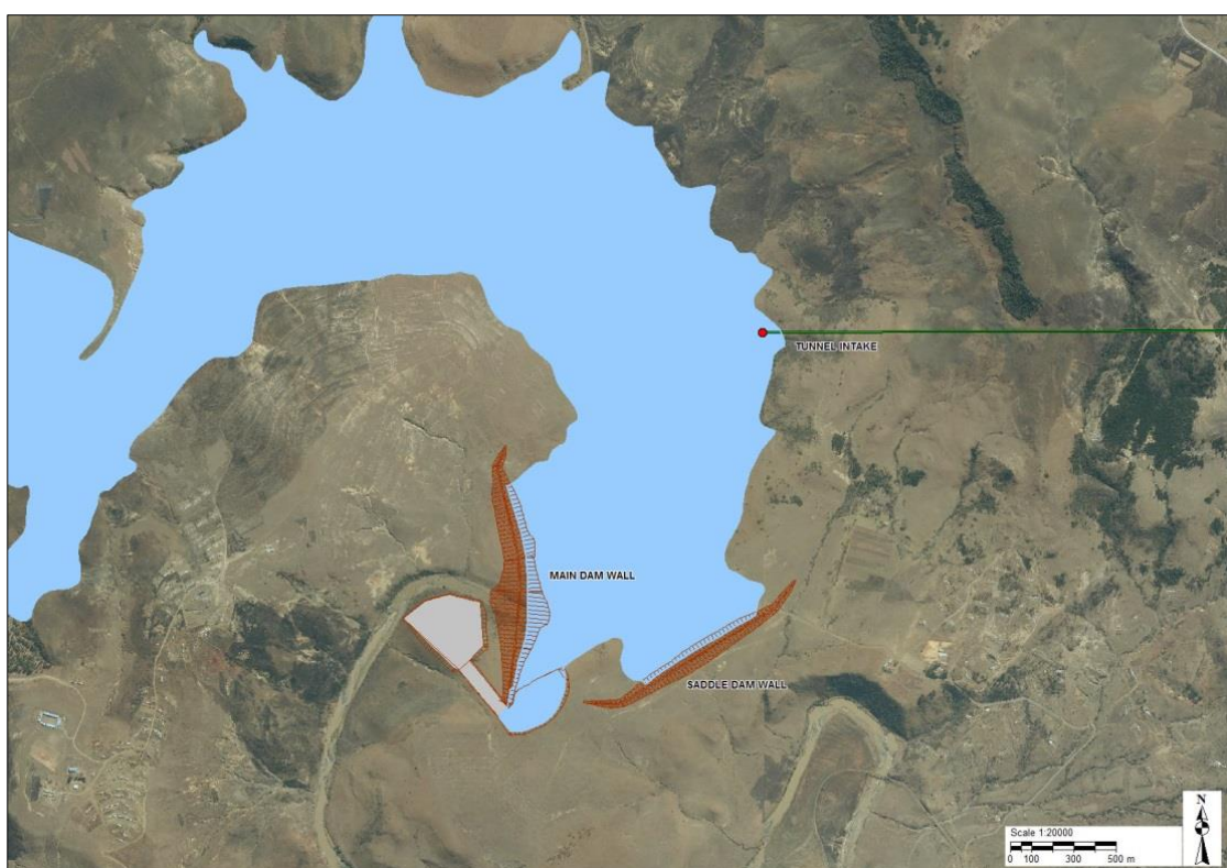
Figure 3.24: Position of the intake structure
